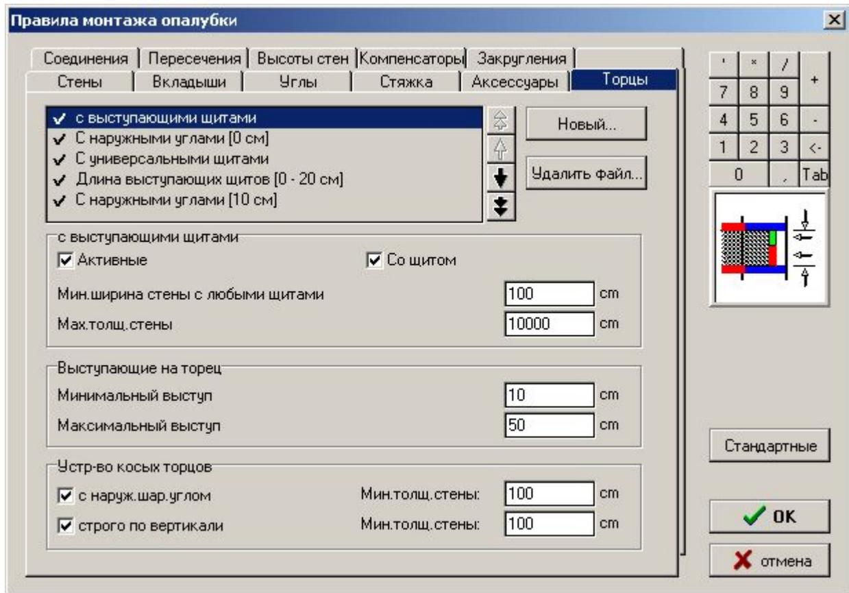
There are different possibilities to arrange formwork at the free wall end (bulkhead). The standard in EuroSchal® is bulkhead with projecting elements. With the button **New** you can enter more possibilities in the list above (depends on form system). EuroSchal® always tries to take the first possibility of the list. If that one is not possible it takes the second possibility and so on, til one possibility works.
