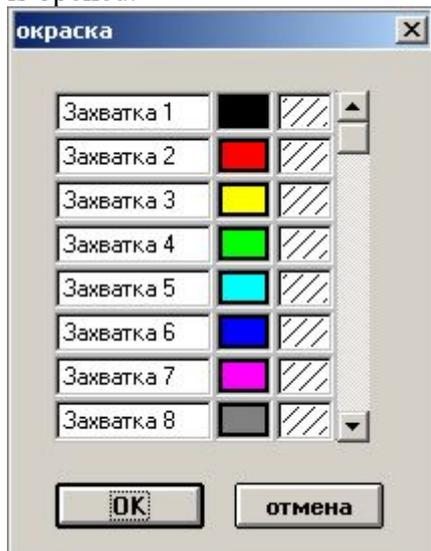
Here you can stipulate the colours and the infill pattern for the walls of the single pours.
