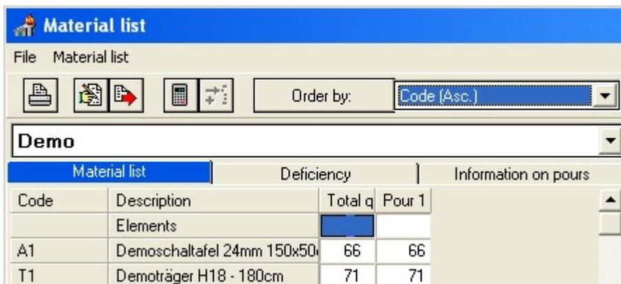
The current displayed manufacturer is shown directly above the table (here „Demo“). With a click on this selection window a list is opened, where all manufacturers are shown which are used in this project. In this list only the manufacturer can be selected whose material is to be shown.
