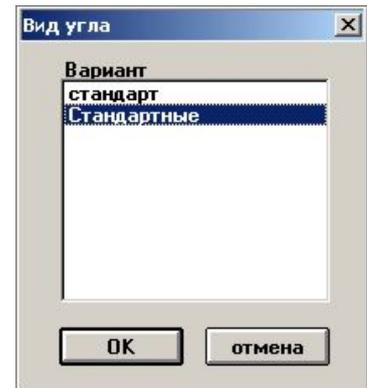
As a standard it is always the item „standard“ active at all corners. This means that the kind of corner shuttering is determined of the formwork setting. If you want to shutter all corners in the same way you do not have to fix different corner variants to all your corners. You can do this simply by changing the formwork setting. You will need this instruction only if you want to shutter a single corner different from the others.
