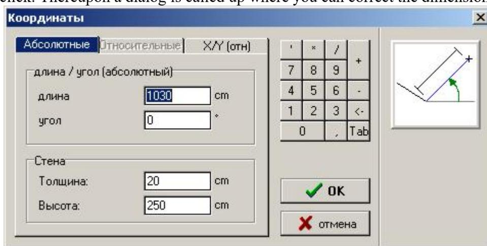
The screenshot shows the 'Координаты' dialog box with the 'Абсолютные' tab selected. The 'длина / угол (абсолютный)' section has 'длина' set to 1030 cm and 'угол' set to 0°. The 'Стена' section has 'Толщина' set to 20 cm and 'Высота' set to 250 cm. A numeric keypad is visible on the right, and a preview window shows a wall being drawn at a 0-degree angle. The 'OK' button is highlighted with a green checkmark.
