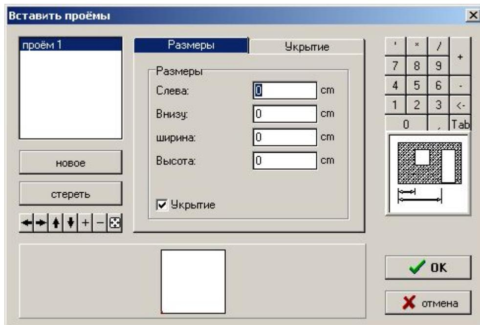
In the left list the openings of this wall are shown. In the area below the side view of the current wall is shown with the entered openings. The marked opening in the top lefthand is shown red.
