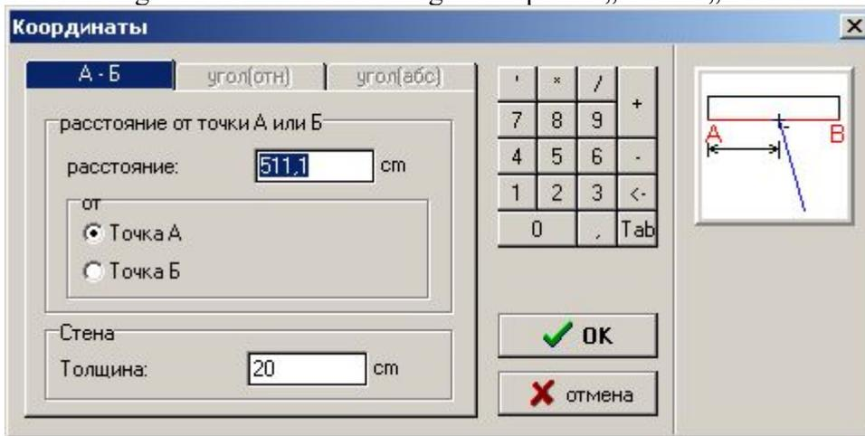
Furthermore a dialog window opens where you can fix the distance of the new wall from „A“ or „B“. This measure is always related to the green drawn line of the wall. In case that the second line is on the wrong side of the line, it can be changed with the instruction “change wall side”.
