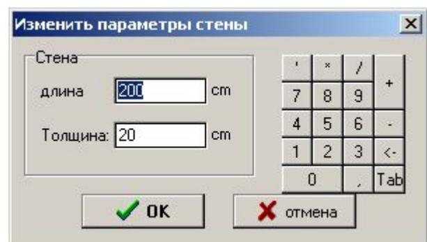
If an input has been made in a dialog, which EuroSchal® cannot assign to the wall, you will be informed. In this case the wall is not changed.
