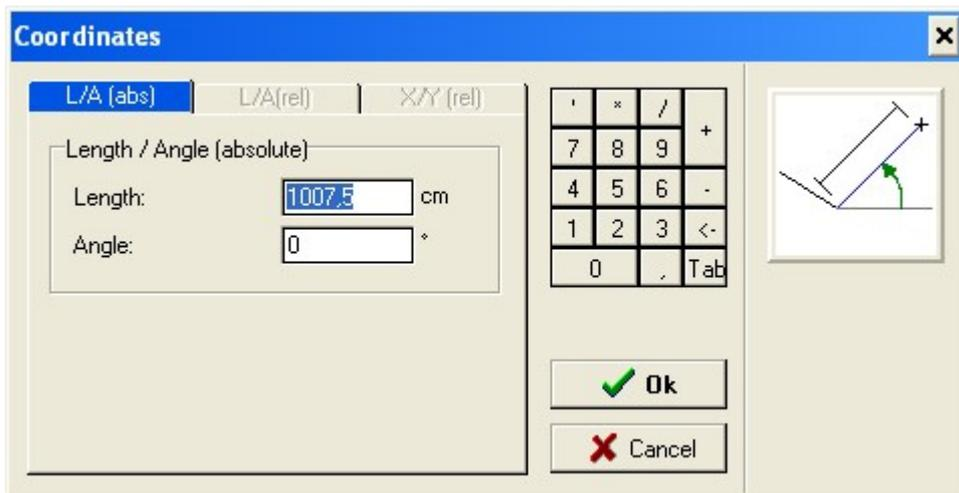
Here you can enter the desired length and angle. The angle is 0° for yoke beams which shows exactly in yoke beam direction of the plane.
