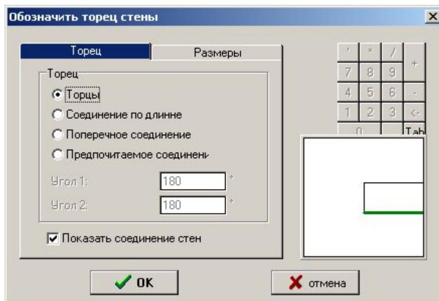
In the register side „wall end“ you can stipulate which kind of end you want to have in this case. „Stopp end“ is a normal wall end. All others name connections at existing walls.
