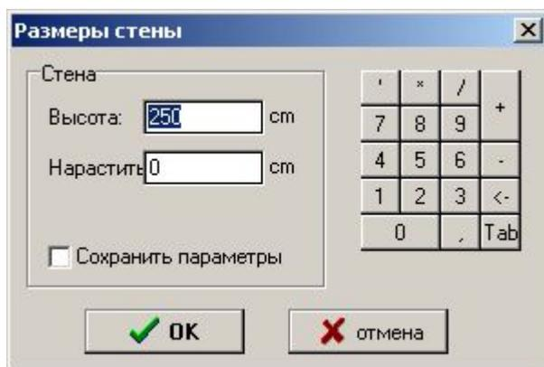
The height is the actual height of the wall. With help of the input field “wall nip” you can enter walls which start from different levels. If a wall has a “nip” of 0cm and the second wall has a “nip” of 50cm, the second wall starts 50cm above the first wall. The wall is measured from this point.
